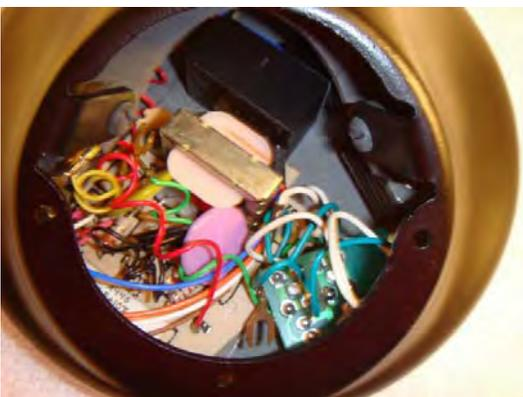
Screw the bottom plate onto the phone body and check that nothing is hitting the internal architecture. Check that the cradle freely springs up and down. Note that the network was mounted at an angle so as to make room for the polarity guard. Place the dial over the opening to make sure it clears. Once assured that everything fits and nothing hits, you're ready to start wiring.
