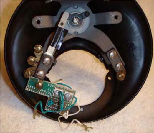
First, use electrical tape to insulate the contacts between the **BK** and **Y** terminals **ONLY**. The **GN** and **W** contacts will be used for the switch hook. The **BK** and **Y** contacts will be used for the transmitter. These later two need to be electrically isolated because the 5.1v Zener must be placed in series for the transmitter. The **Y** terminal screw will also be used to mount the polarity guard.
