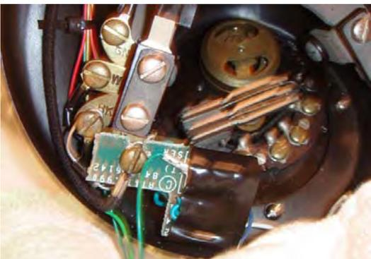
Mount the polarity guard to **Y** and the handset BLACK wire.
