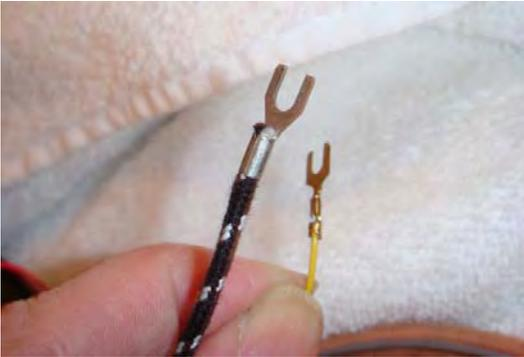
The handset White attaches to the AE network Yellow. The dial "W" is not used. "Popping" in the receiver is not an issue with a Rotatone installation because pulse signals are no longer sent into the line.
