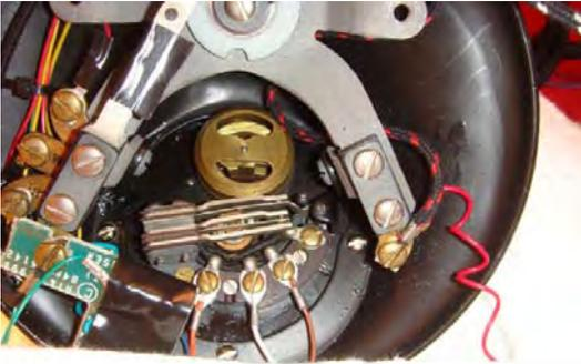
Attach the Rotatone wires to the 2AB dial:
